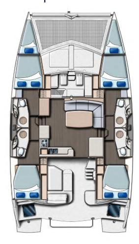
The Leopard 44 is available in either a 3 cabin, 3 head version, or a 4 cabin, 4 head version. Both layouts offer the option of additional storage, berth, or head in the forward hull.
